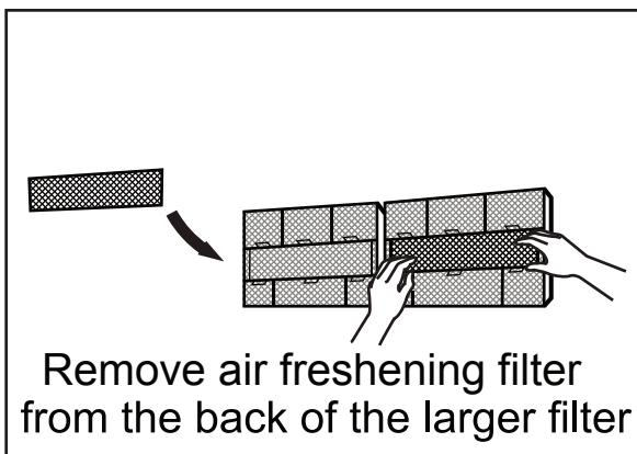
**Remove air freshening filter from the back of the larger filter**
