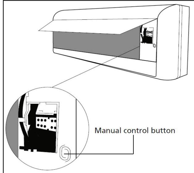
**Note:** The manual button is intended for testing purposes and emergency operation only. Do not use this function unless absolutely necessary. To restore regular operation, use the remote control to activate the appliance.
