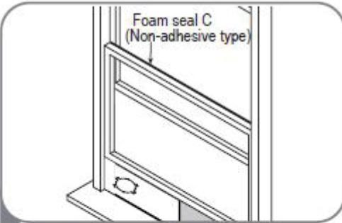
3 Cut the non-adhesive foam seal C strip to match the width of the window. Insert the seal between the glass and the window frame to prevent air and insects from getting into the room.
