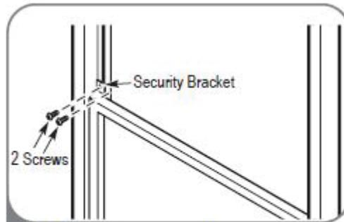
4 If desired, install the security bracket with 2 screws as shown.
