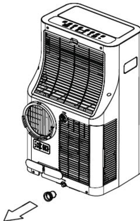
During the DRY mode, you may wish to set up the continuous drain option so that the unit will automatically drain collected water.
