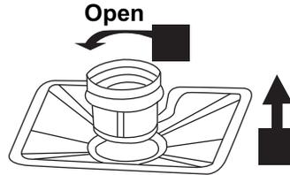
**Step 1.** Counter-rotate the fine filter.
