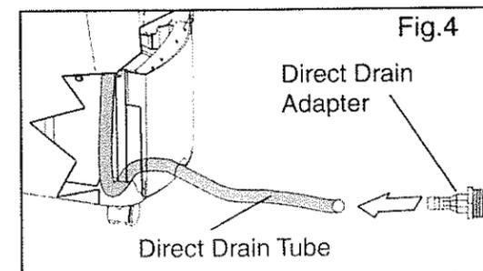
**Please Note:** Remember to reverse the above direct drain instructions when relocating the unit to a location where continuous drain is not possible. Failure to replace and recap the direct drain hose may result in flooding of the immediate area.
