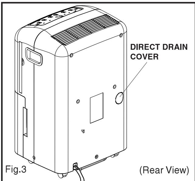
2. Cut drain hose to required length. (to suit your needs) You do not need any fittings on either end of the drain hose. Insert one end the of garden hose directly into the direct drain opening. (See Fig. 4)
