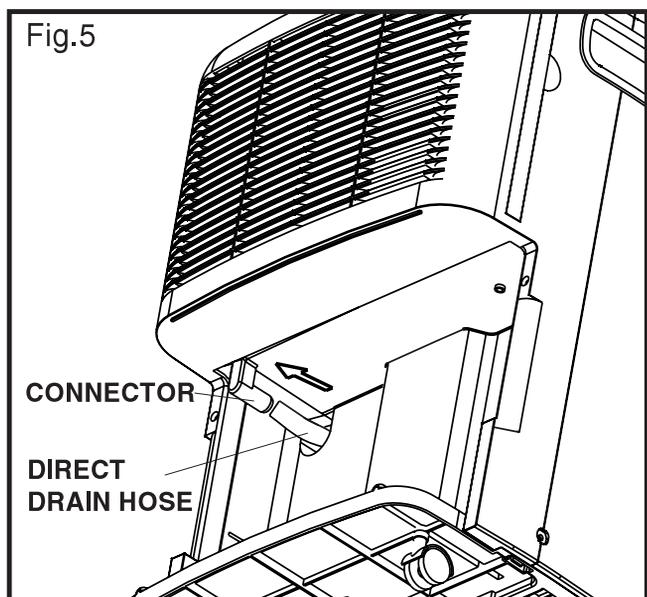
4. Re-install the water tank, making sure the water full light turns "off". If the light remains on, the tank has not been properly installed. The water tank must always be installed inside the cabinet whenever the direct drain option is being used.
